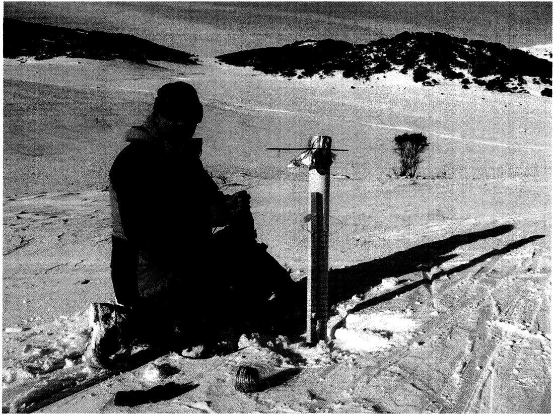
Figure 5.2 Snow tube with a one metre extension fitted. Snow surface is approximately 120 cm above the ground.
